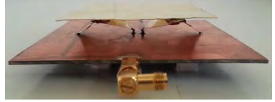
Fig. 1. Topology (left) and photograph (right) of a low-profile, ultra-wideband antenna developed in this project. This antenna has the lowest profile of all UWB antennas reported to date that radiates like a vertically-polarized monopole and have very compact dimensions. The antenna has an overall bandwidth of 4:1.
