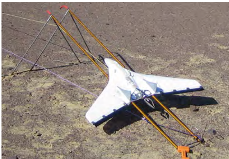
Figure 1. DataHawk on launch rails during field measurements in Paracas, Peru in July 2011.
