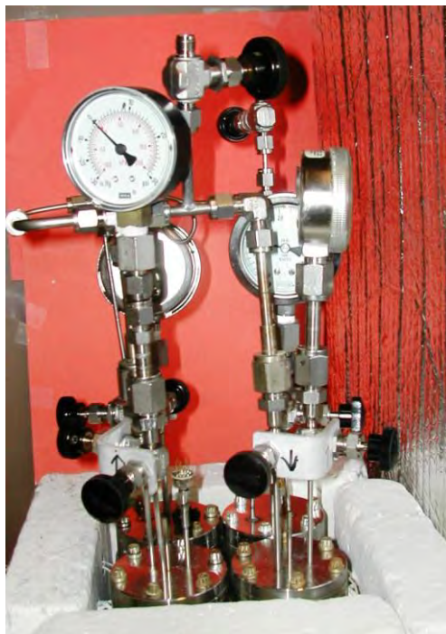
Figure 10. Matrix calorimeters in their heating block with the gas/vacuum manifold attached.
