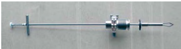
Fig. 2.2. Sample manipulator option for turning samples in-situ, without opening the chamber.
