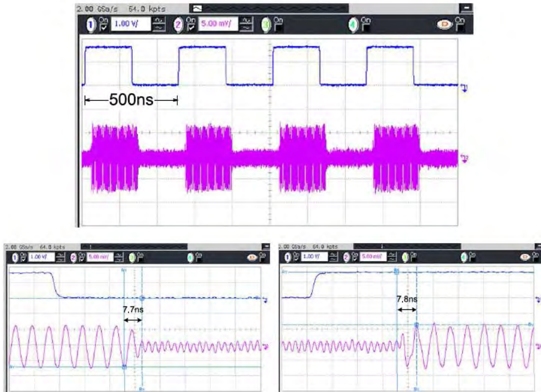
Figure 58: (a) Measured 2MHz hopping between Channel 2 and 6 at output 2. (b) A closer look at the transition from channel 2 to channel 6. (c) A closer look at the transition from channel 6 to channel 2.
