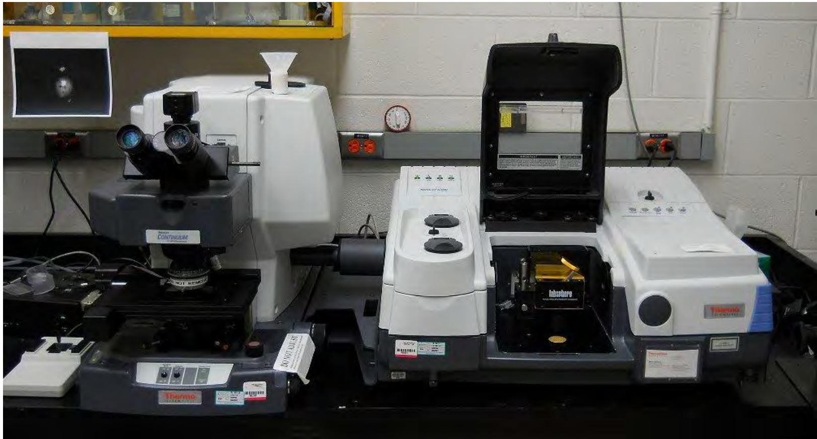
Thermo-Nicolet 6700 FTIR and Continuum Microscope Labsphere integrating sphere in sample compartment at right
