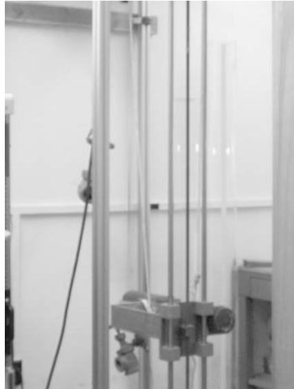
Figure 1. Photograph of traversing setup, with detector and radiation source in place.
