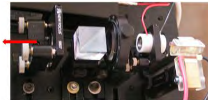
Figure 6 – New high pulse energy Q-switched MO
