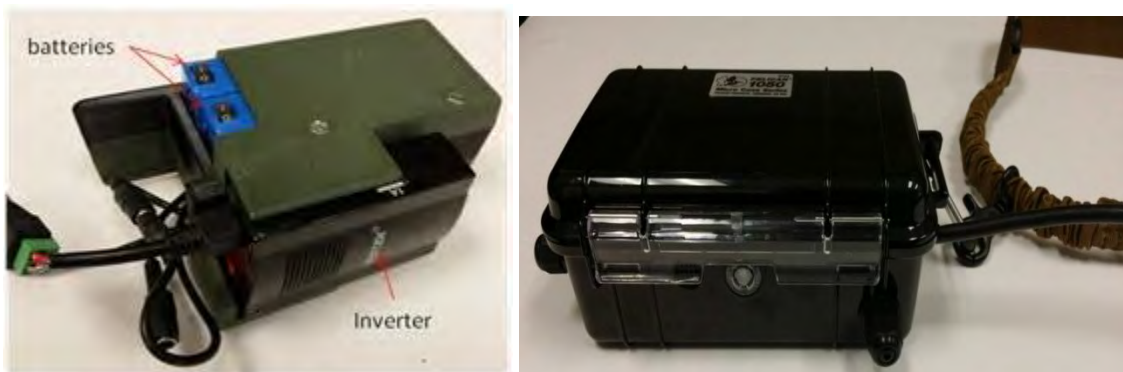
Figure 44 – Polymer Li-ion battery for powering the burst laser system
