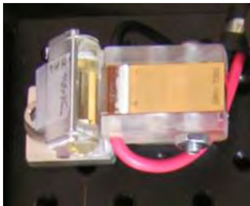
Figure 10 – Photograph of the PA laser head
