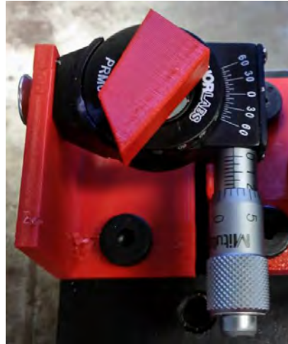
Figure 23 – 3D printed model of PB rotating mount
