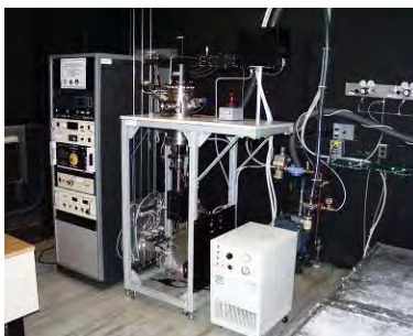
Figure A.33. 1.5 kW Diamond Deposition System
