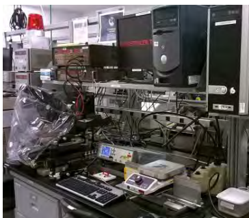
Figure A.49. Curve Tracer Test System
