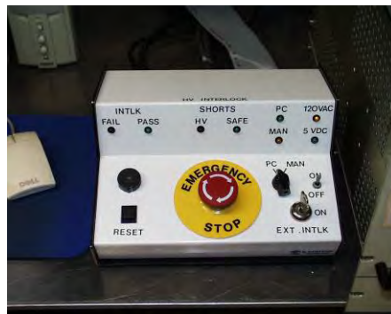
Figure A.48. Safety Interlock System
