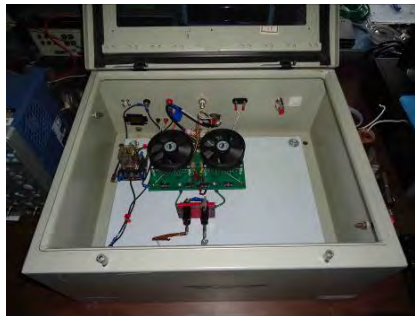
Figure A.64. Safety Interlock Controlled Test Fixture
