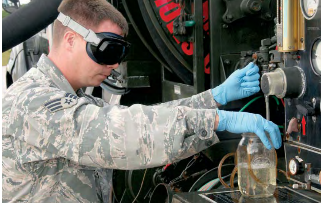
Air Force Senior Airman Ben English drains fuel from an R-12 refueling truck at Andersen Air Force Base, Guam, to sample it prior to use. Warfighters get the jet fuel they need through contracts executed by the Defense Logistics Agency.
