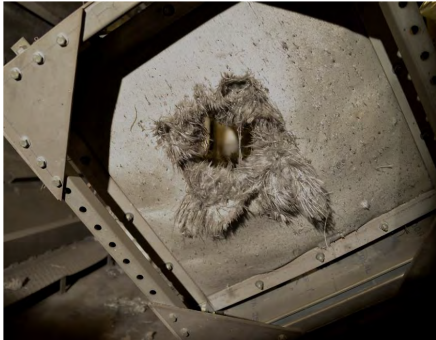
Front side of 1 st bumper. Note that some fiberglass has ejected up range.
