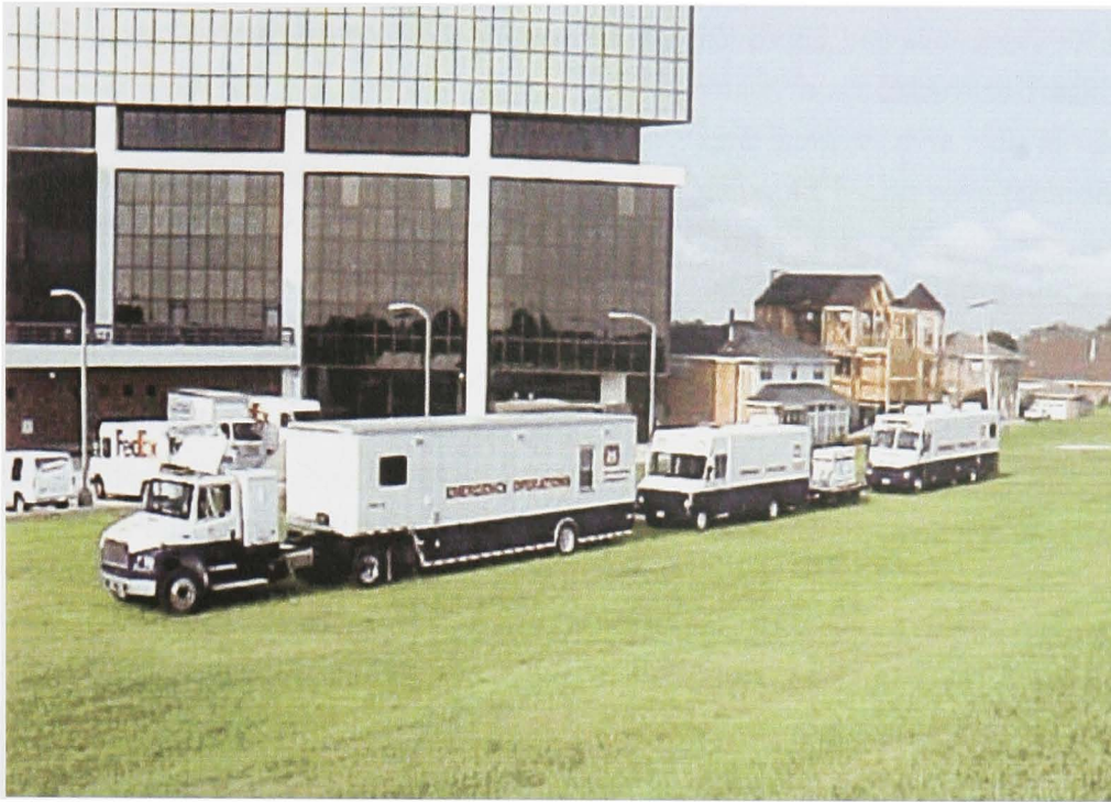
Mobile District DTOS vehicles. The tractor-trailer unit is the ECCV, the second vehicle with the antenna unit is the ESSV, and the last unit is the ETOC.
