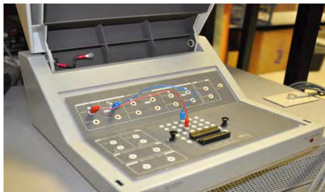
Figure 91. Test fixture used for performing automated electrical measurements
