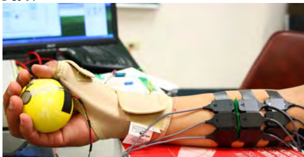
Figure 2: Force sensitive Resistor and Thumb Restrain
