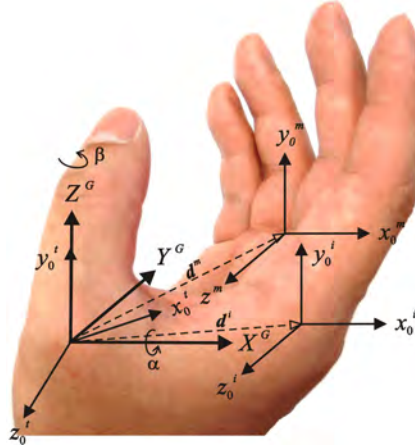
Figure 3: Relationship between Global Coordinate and Local Coordinates: Local coordinate x^t - y^t - z^t of thumb can be reached by rotating through angles \alpha and \beta to X^G and Y^G of global coordinate, subsequently. Local coordinate x^i - y^i - z^i of index finger can be obtained by rotating through angle \alpha to X^G and then translating a vector \mathbf{d}^i of the global coordinate.
