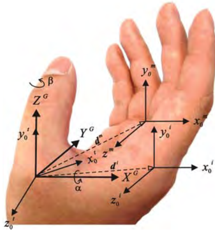
Fig. 1. Relationship between Global Coordinate and Local Coordinates: Local coordinate x^t - y^t - z^t of thumb can be reached by rotating through angles \alpha and \beta to X^G and Y^G of global coordinate, subsequently. Local coordinate x^i - y^i - z^i of index finger can be obtained by rotating through angle \alpha to X^G and then translating a vector \mathbf{d}^i of the global coordinate.
