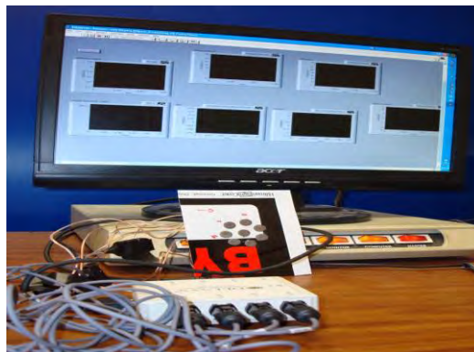
Fig. 3.1.1(b): Array Sensors Tested on NI LabVIEW™.
