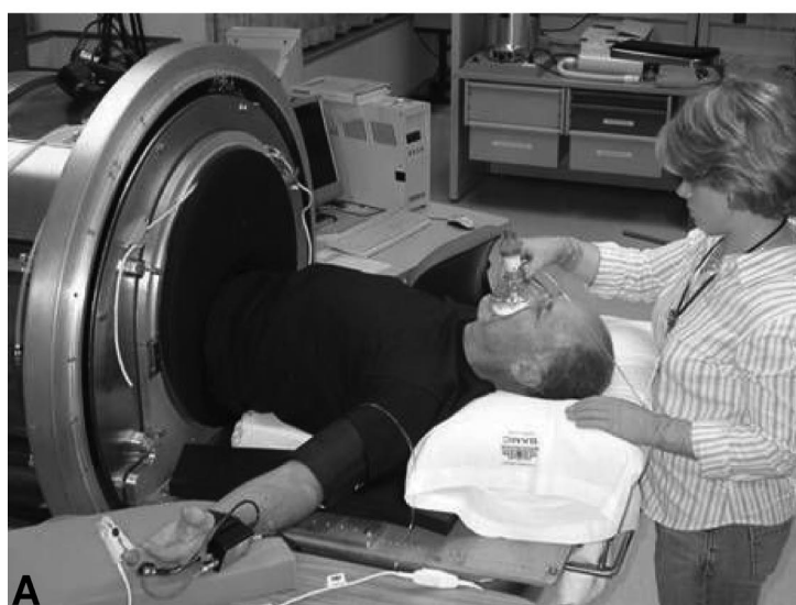
Figure 1. Subject in the lower body negative pressure (LBNP) device breathing through an impedance threshold device (A) and the LBNP protocol (B). Bottom abscissa indicates Cardiovascular Collapse Index corresponding to integrated product of time and LBNP level.
