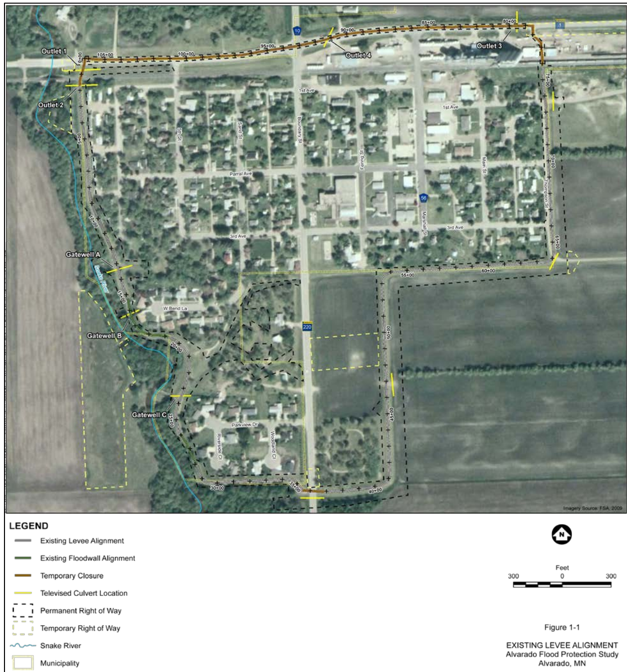
FIGURE 2: LAYOUT OF THE EXISTING LEVEE SYSTEM
