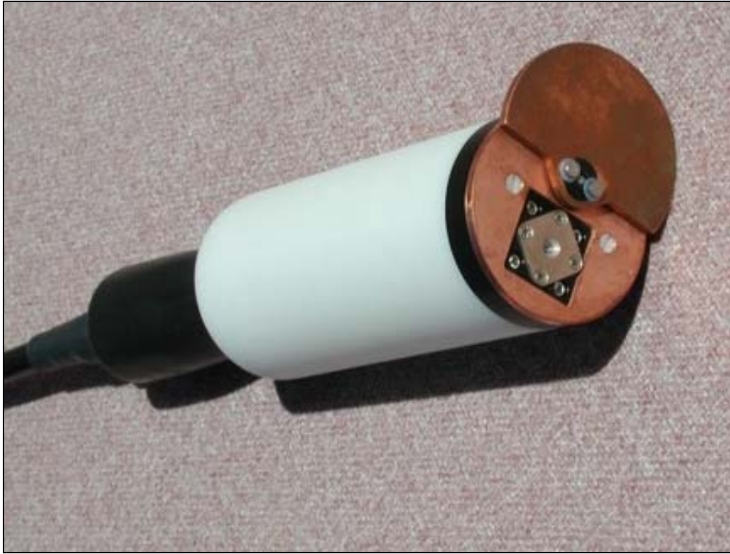
Figure 2. HydroRad fiber-optic light collector with new integrated HydroShutter. The HydroShutter covers the optics of the light collector with a copper plate to prevent bio-fouling. During sampling, the plate is rotated out of the way of the optics. Long-term mooring deployments have demonstrated that this technology keeps the optics free of fouling for over three months in highly fouling environments.
