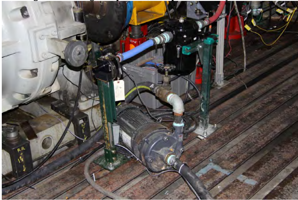
Figure 6: Testing Components, Pump and Blow-by Meter
