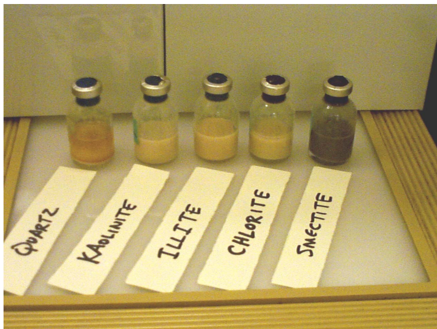
Figure 1. Set of FeOx-reducing enrichments grown on acetate. Note the obvious difference in color due to differences in the transformation of iron. FeOx was least reduced (still mostly orange in color) when present with quartz and most reduced (forming a black color) with smectite.
