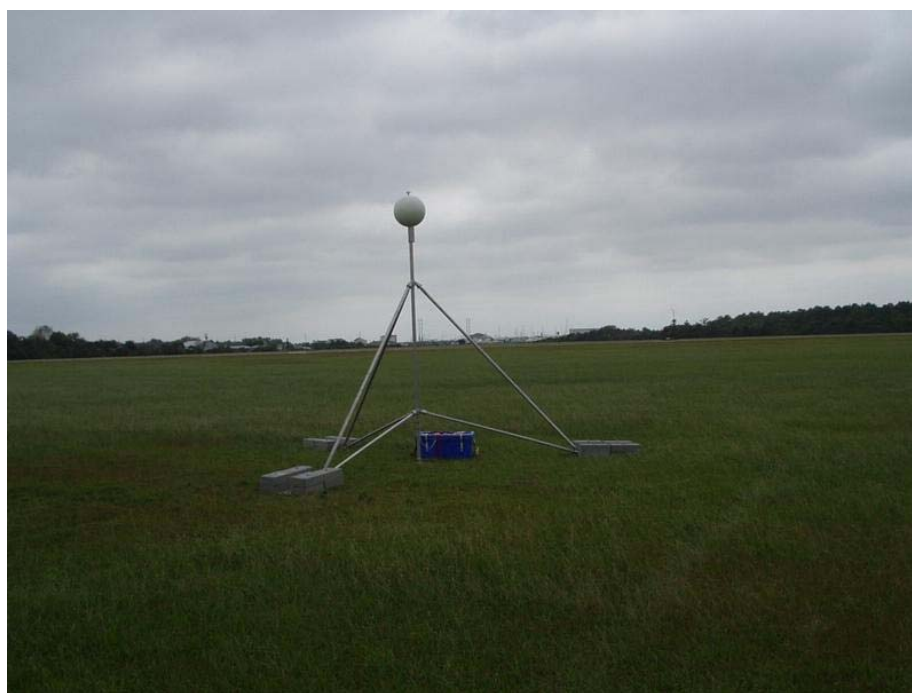
Fig. 3. Deployed ET probe on 17 September 2003 near Beaufort, NC. Hurricane Isabel made landfall the following day.
