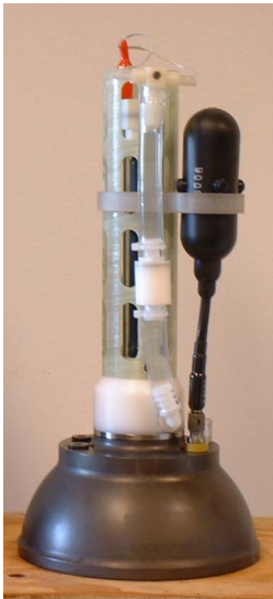
Figure 1. An Webb/Apex float head, showing a SeaBird CTD unit and a low-frequency hydrophone capable of receiving RAFOS transmissions.
