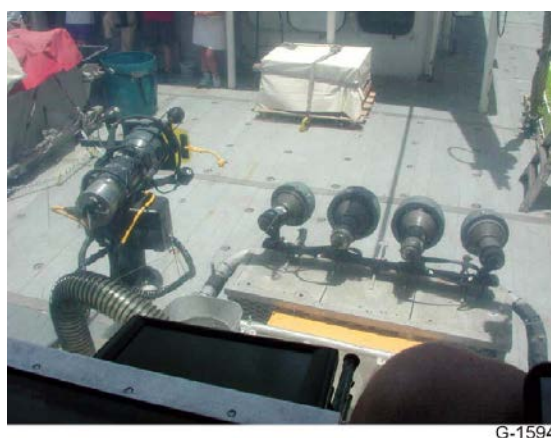
Figure 1. View from inside the Johnson-SeaLink sphere showing the HMI lights mounted far forward on the tiltable lid of the work basket. The two inner lights are fitted with filters that transmit blue light, while the outer two are fitted with filters that transmit ultraviolet. The two pairs can be illuminated separately. To the left is the JSL video camera fitted with a yellow barrier filter for imaging blue-light stimulated fluorescence.
