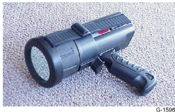
Figure 3. Underwater Kinetics Light Cannon high intensity discharge dive light fitted with a custom interference filter. The light is an effective illumination source for fluorescence exploration and close-range documentation by videotape.
