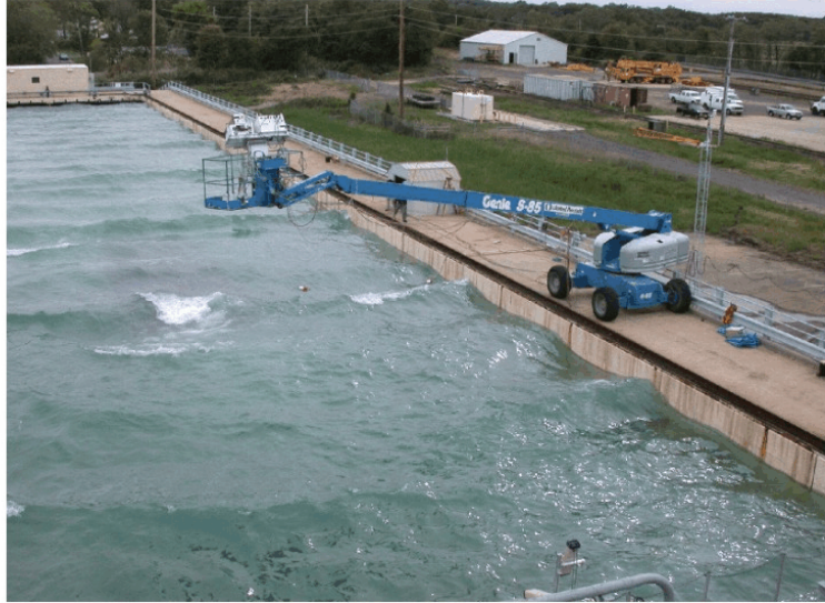
Figure 1: Overview photograph of the OHMSETT wave basin showing the radiometers, mounting crane, and breaking waves generated on the shoal.
