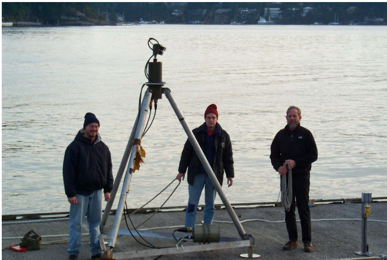
Figure 1. The PAL tripod just prior to deployment off the outer breakwater of the Friday Harbor Laboratories pier [The rotator and transducers are at the top; other electronics are in the side-mounted canister along the base. Helping with the deployment are (left to right) Shawn Shellito, Liko Self and Pete Jumars]
