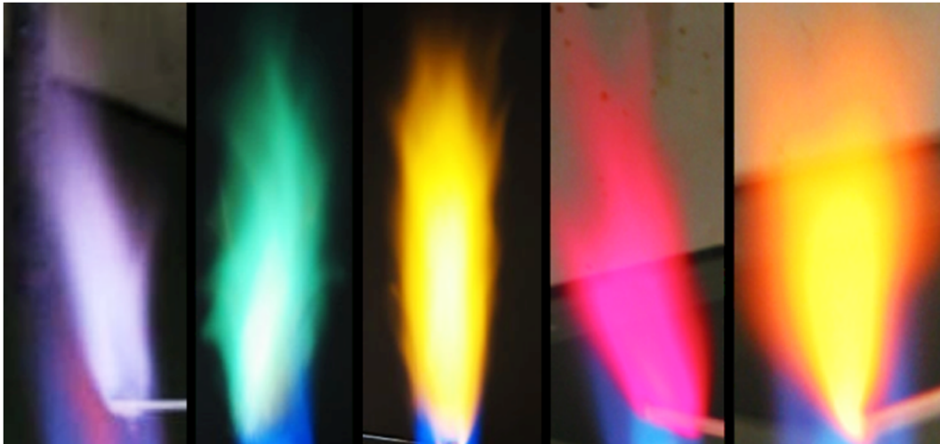
salts of arsenic, copper, sodium, lithium, and calcium burn within a flame
