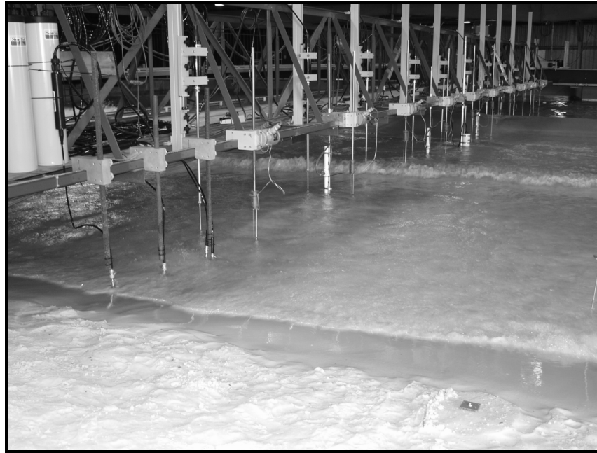
Figure 1. LSTF showing waves, the instrumentation bridge, wave gages and ADV's.
