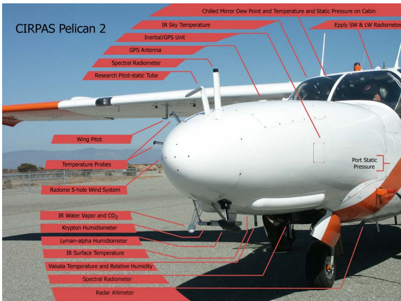
Figure 1 Main meteorological and turbulence instrumentation on the CIRPAS Pelican aircraft during the summer 2003 CBLAST-Low.
