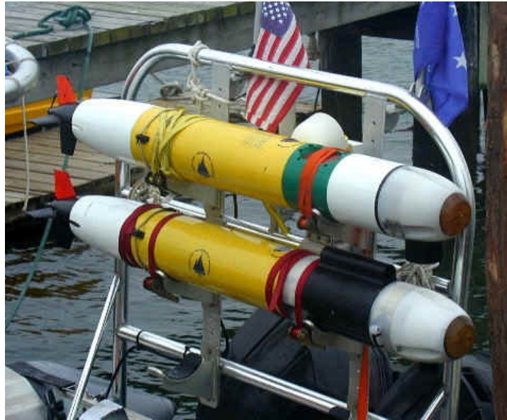
Figure 1. ADCP and Bioluminescence REMUS vehicles prior to deployment
