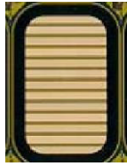
Figure 2. Photo of 3.5 cm 2 Si SGTOs. The anode contact is on the bottom side, and the gate and cathode contacts is on the top side.
