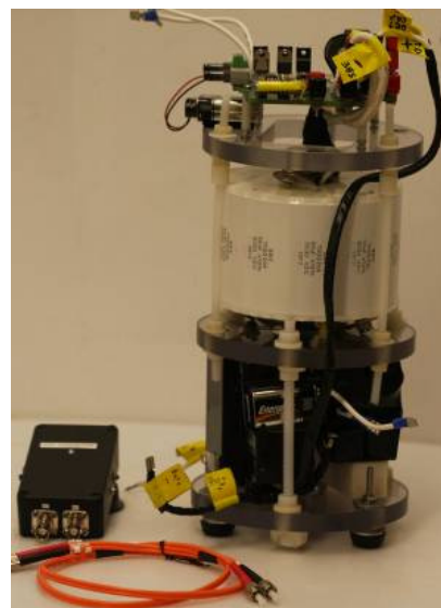
Figure 1. CSS and CTS stand-alone apparatus as used in laboratory testing with fiber-optic transmitter.
