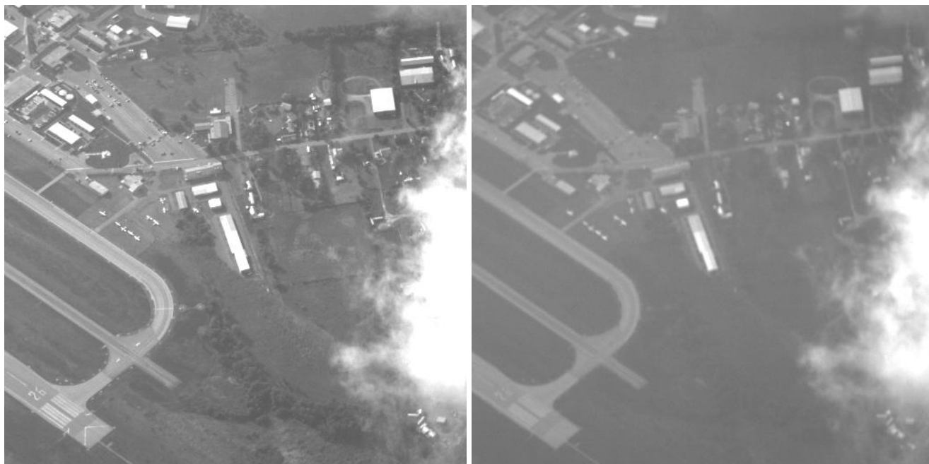
Figure 1. AROSS-MC Imagery from the test flight on Sep 11, 2003 over the Martinsburg, WV airport, the left frame is the red channel and the right frame is the blue channel. [images of runway and hangars, left image has greater resolution than right image]
