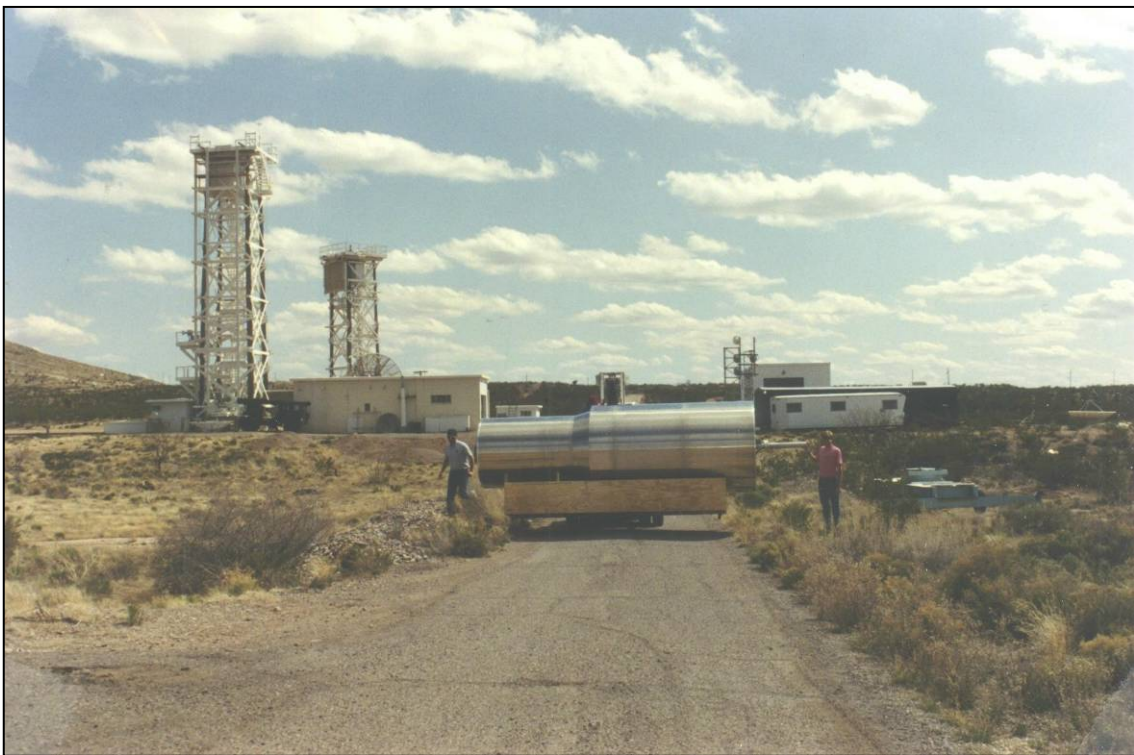
Figure 6-2. Pegasus bulbous fairing mockup prior to antenna testing (PSL).
