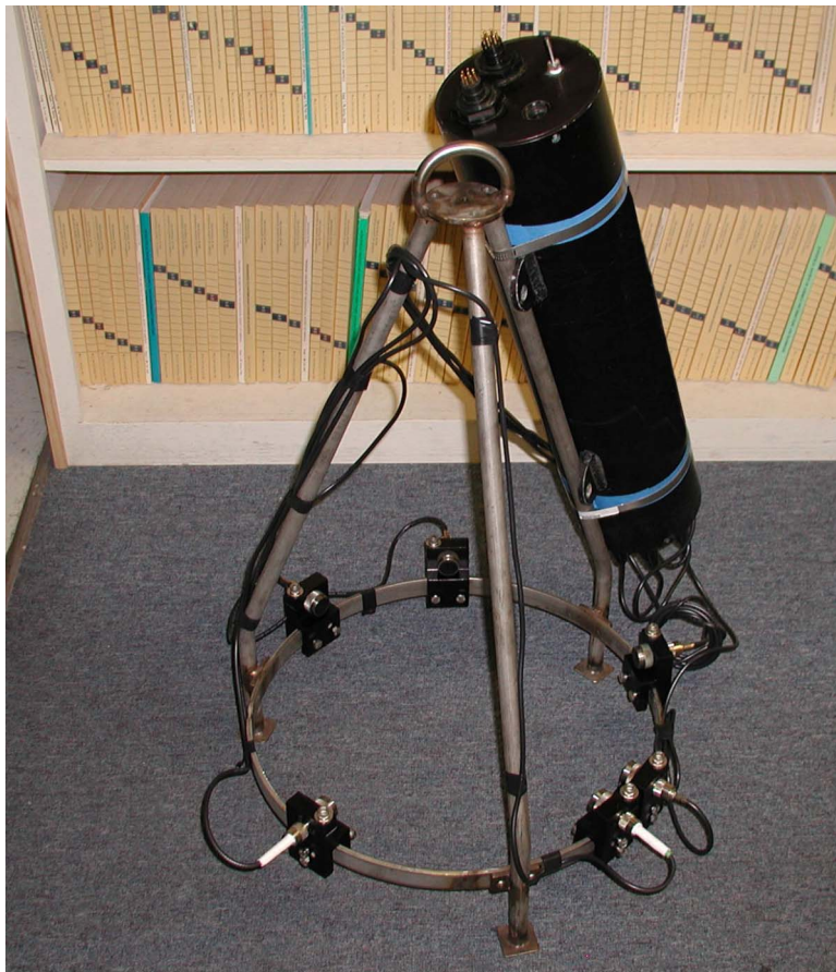
Figure 3: A circular frame holds several broadband transducers aimed at the center of the frame. The long black cylinder is a pressure case for electronics. This configuration uses two transmitting transducers in order to cover a wide frequency band (bottom right). Pulses are directed across the diameter of the measurement plane. Multiple receiving transducers are located at known, adjustable, angles in the horizontal plane and are used to intercept echoes when one (or more) scatterer is detected in a very small volume in the center of the circle formed by the frame.
