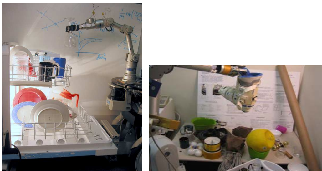
(a) Our robot unloading items from a dishwasher. (b) Grasping in cluttered environment with a multi-fingered hand
