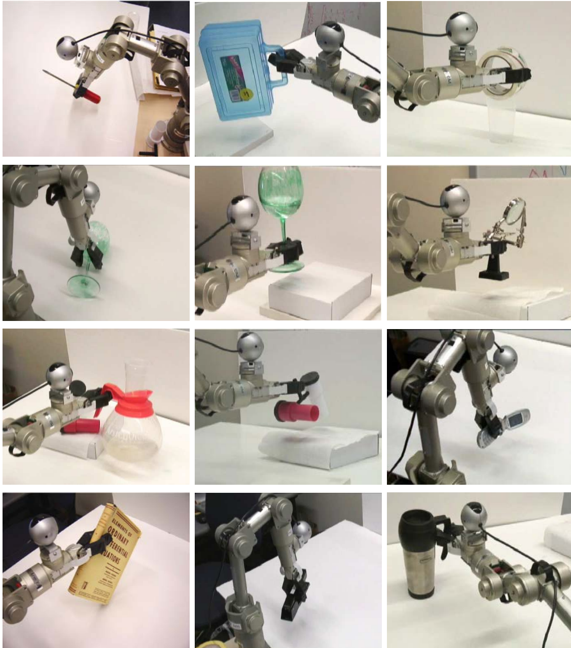
Figure 5.11: The robotic arm picking up various objects: screwdriver, box, tape-roll, wine glass, a solder tool holder, coffee pot, powerhorn, cellphone, book, stapler and coffee mug. (See Section 5.7.2.)
