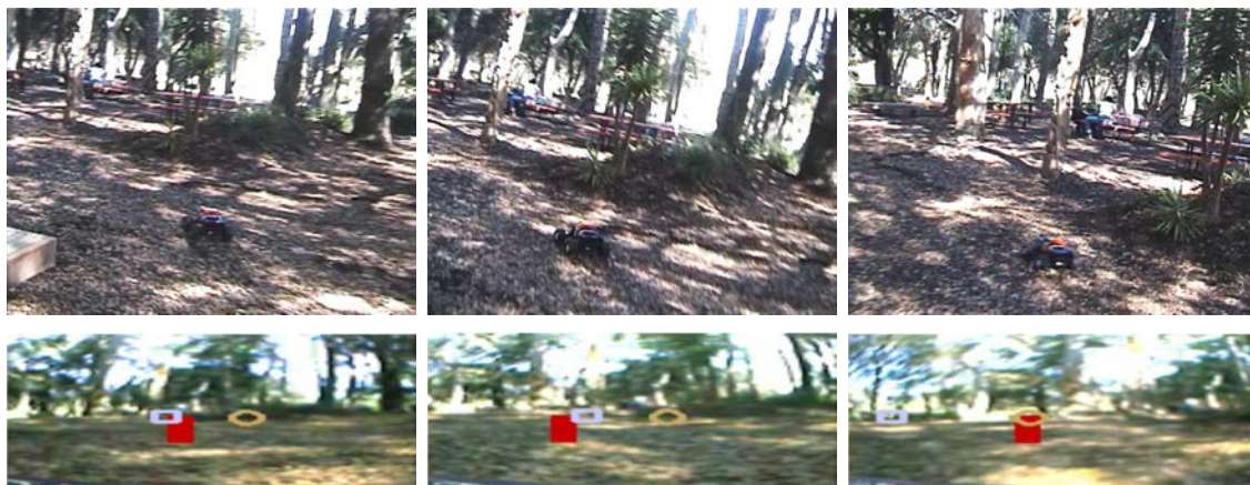
Figure 4.8: An image sequence showing the car avoiding a small bush, a difficult obstacle to detect in presence of trees which are larger visually yet more distant. (a) First row shows the car driving to avoid a series of obstacles (b) Second row shows the car view. (Blue square is the largest distance direction. Red square is the chosen steering direction by the controller.) (Best viewed in color)
