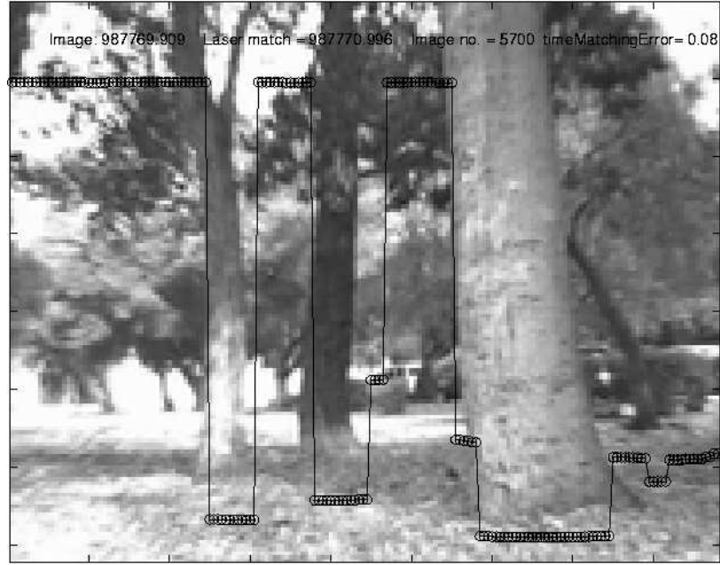
Figure 4.2: Laser range scans overlaid on the image. Laser scans give one range estimate per degree.
