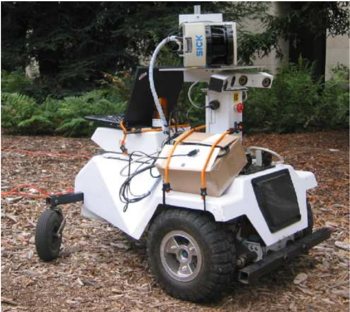
Figure 2.18: The custom built 3D scanner for collecting depthmaps with stereo image pairs, mounted on the LAGR robot.
