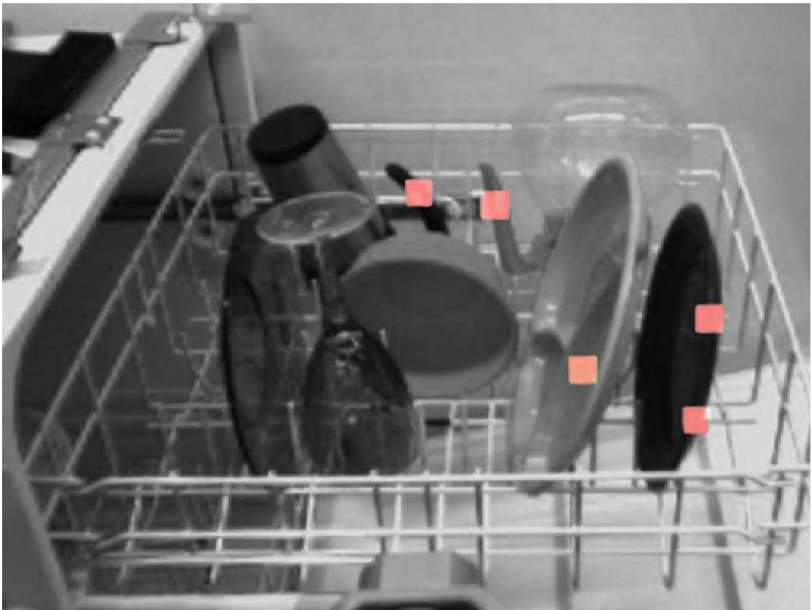
Figure 5.13: Grasping point detection for objects in a dishwasher. (Only the points in top five grasping regions are shown.)
