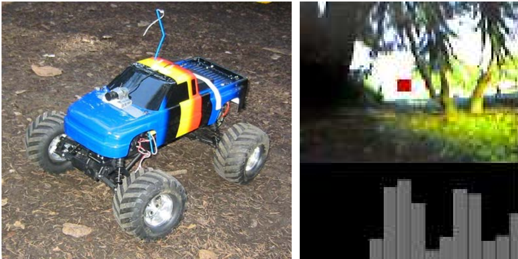
Figure 4.1: (a) The remote-controlled car driven autonomously in various cluttered unconstrained environments, using our algorithm. (b) A view from the car, with the chosen steering direction indicated by the red square; the estimated distances to obstacles in the different directions are shown by the bar graph below the image.
