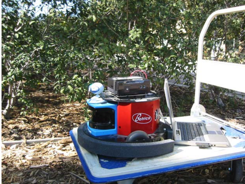
Figure 4.3: Rig for collecting correlated laser range scans and real camera images.
