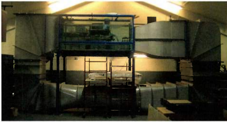
Figure 8: Circulating water channel with platform and instrumentation
