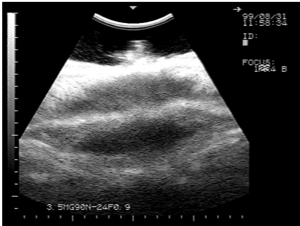
2. Ultrasound image in diatom mat area, August 23, 1999. Image is essentially cross section through sediment. Note presence of animal burrows in upper left of image. Tick marks are 1 cm.
