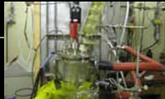
A Modified Decomposition Hydrolysis System is being developed to allow safe and effective disposal of explosives residue found on range scrap
