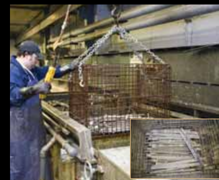
Three HAP-free strippers were applied to various ground vehicle parts at ANAD to determine potential performance and cost benefits. The basket shown contains steel locking plates, which were completely stripped of their MIL-C-22750 coating by a water-based, acid-activated stripper at a rate comparable to the current solvent.
