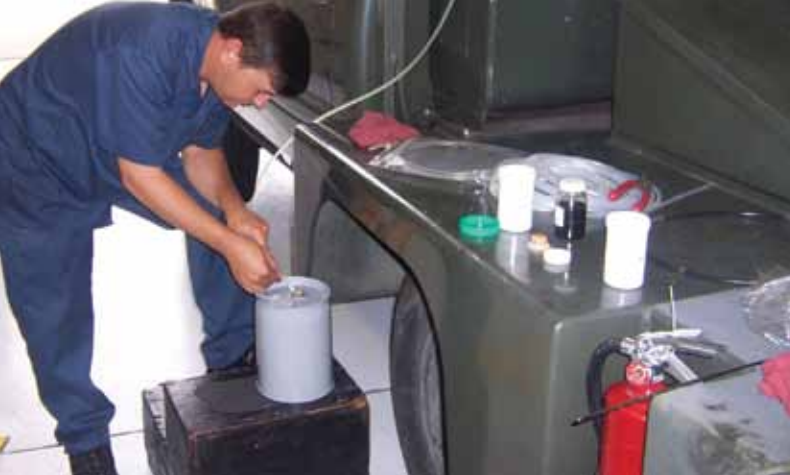
The demonstration and validation of biodiesel use involves sampling of fuel quality within tactical vehicles as well as storage facilities and monitoring of maintenance records. Testing is done under a wide range of operating conditions.
