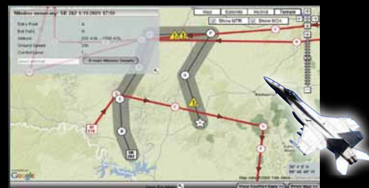
JLLDT interface clearly warns pilots of potential conflict on their scheduled missions. It includes yellow warning triangle icons on the map and in a summary box with details. The tabular interface also displays the mission conflict data in a very easy to use user interface.
