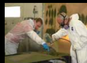
Single Component Chemical Agent Resistant Coating (CARC) transitioned to Anniston Army Depot, AL, and Fort Wainwright, AK; Water Dispersible CARC transitioned to Fort Wainwright, AK
