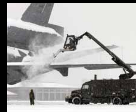
The NDCEE conducted material compatibility testing of anti-icing fluids – enabling the use of drop in replacements that will reduce the use of propylene glycol, improve the efficiency of aircraft deicing operations, and enhance military readiness.
