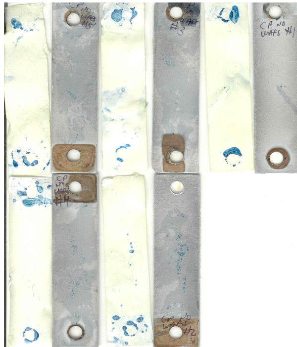
Figure 5-4: Porosity test of hard chromium from tank without Fumetrol® 140 (Cherry Point)
