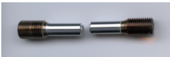
Figure 5-3: Notched Round Bar for Hydrogen Embrittlement Testing
