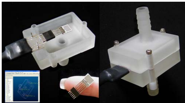
Figure 6. SLA-Fabricated Sensing Element Enclosure Made with WaterShed™ 11120
