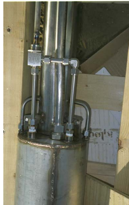
Figure 7. Bottom container of the LRDP housing the sensor systems.
