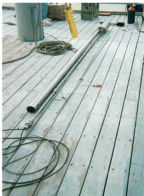
Figure 5. In-tank portion of the LRDP system for a bulk UST with vertical walls.
