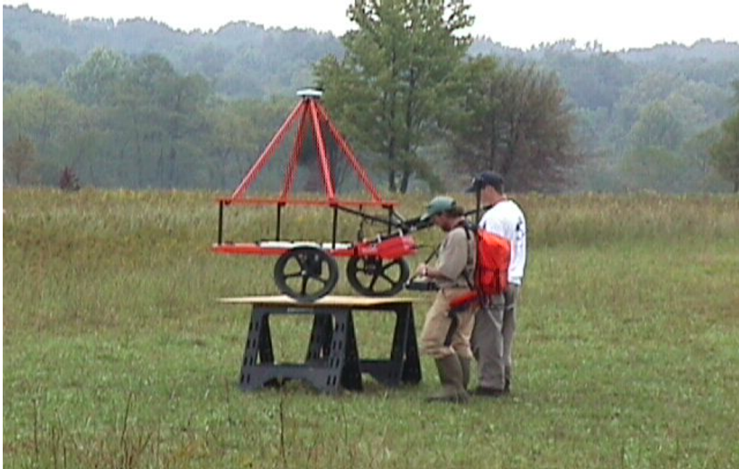
Zeroing of the EM-63 before surveying
