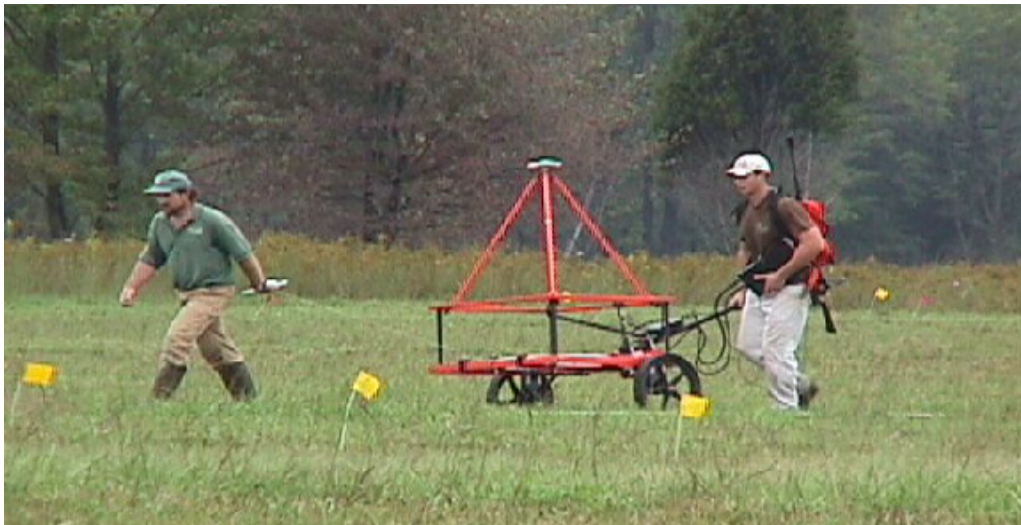
Figure 2: Traversing Grid 3 with the EM-63 (Ropes at 2m intervals)
