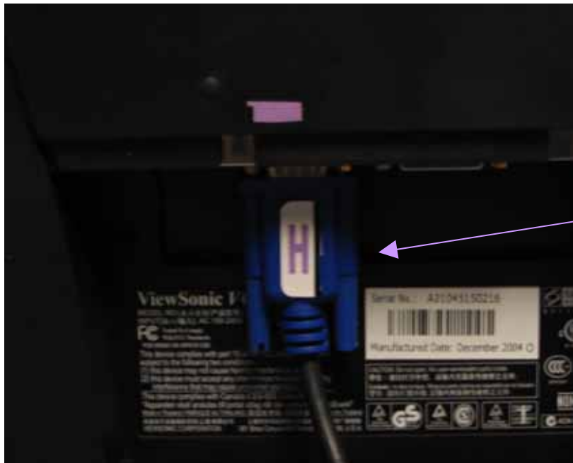
Monitor Line in Back of Monitor
