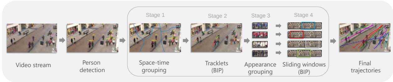
Figure 2: The proposed single-camera processing pipeline from detections to trajectories. One more inter-camera stage aggregates trajectories into identities.
