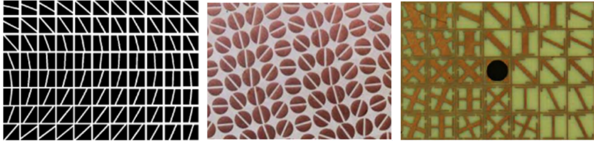
Figure 2. Examples of previous anisotropic surfaces include the original holographic tensor impedance surface created by the author (left), a similar structure studied by Stefano Maci (center), and another variant studied by Tony Grbic (right).
