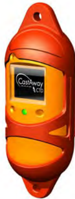
Figure 8. CastAway CTD Utilized for Instantaneous Profiles of Temperature, Salinity, and Sound Speed
