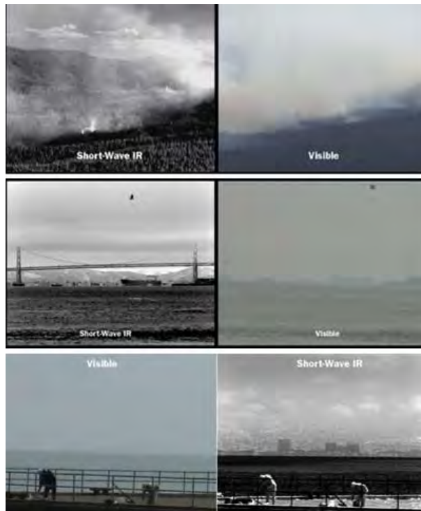
Figure 3. Scattering Effects of Smoke, Fog, and Atmospheric Obscurants in the Visible and Infrared Bands
