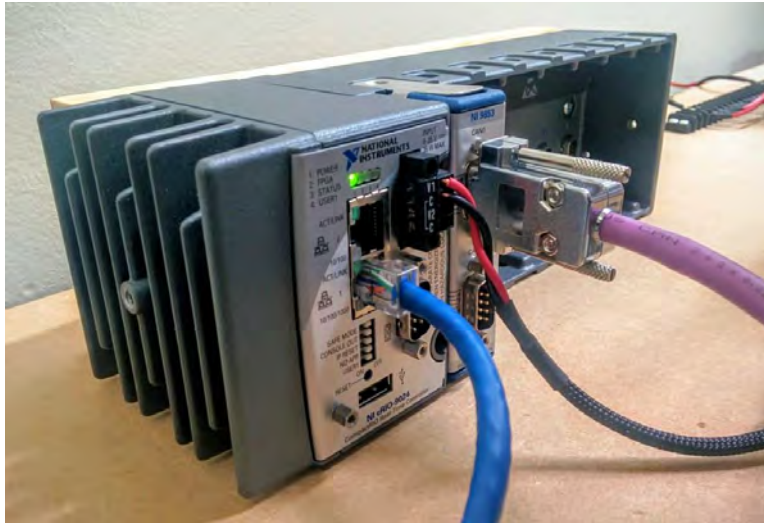
Figure 17. NI cRIO 9024 Real-Time Controller, cRIO 9114 Reconfigurable Chassis, and 9853 2 Port, High-Speed CAN Module
