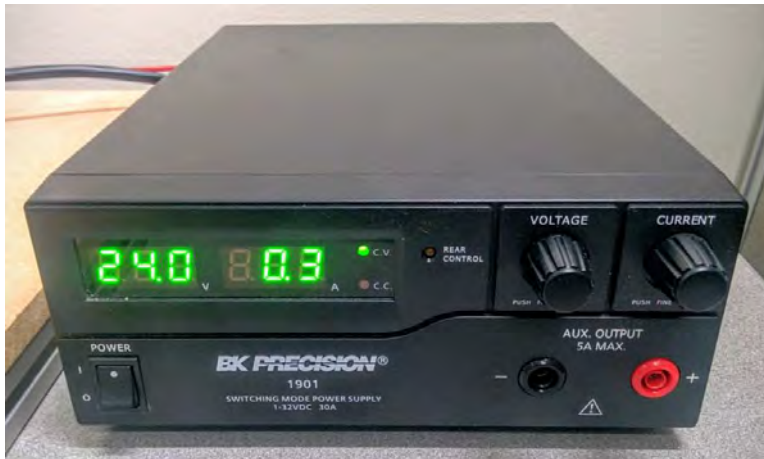
Figure 15. BK Precision 1901 Switching Mode Power Supply
