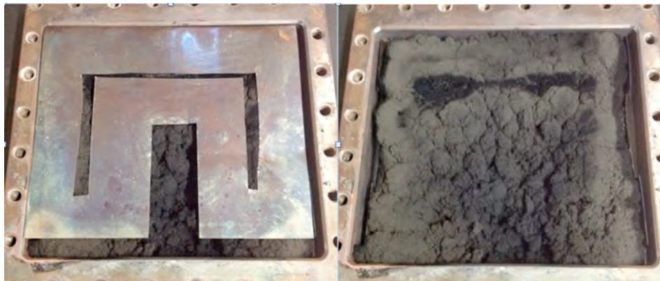
Figure 35. Left image shows Foil Deflector THREE's experiment after opening of the main. Right image shows the CFF generated during the process.
