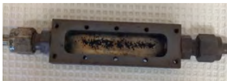
Figure 9. Early CFF experimental mold (dimensions of 0.5 x 0.344 x 2.25 inches) shown with 0.02 grams of palladium distributed within the chamber.
