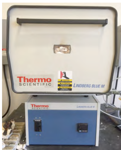
Figure 5. LindBerg Blue M model BF51442C furnace shown from the front with chamber door closed and window packing material in place.
