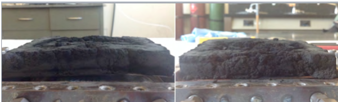
Figure 45. Left image shows a forward view of the CFF block generated during Foil Deflector SIX's experiment and placed atop the main chamber after removal. Right image shows a rear view of the results.
