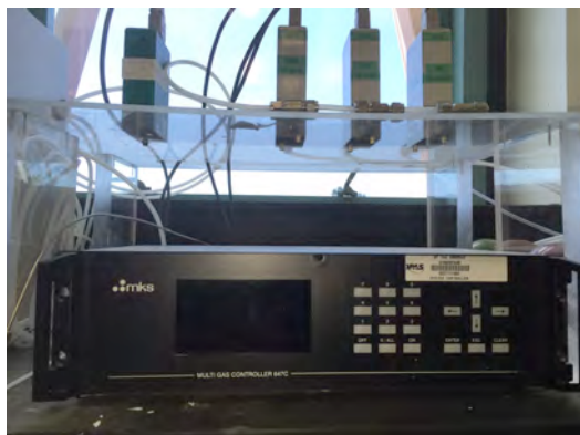
Figure 7. MKS mass flow controller (model MKS 647a).
