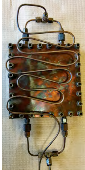
Figure 10. Increased chamber inlet length shown attached to the scaled mold.
