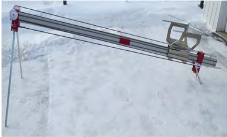
Figure 3.4: AVA Bungee Launcher, from [25]
