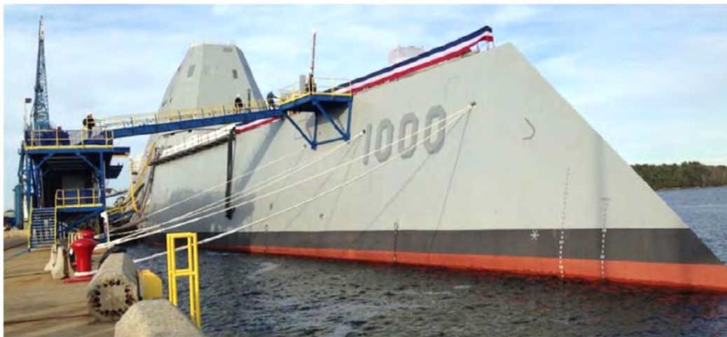
Figure 4. Tumblehome Hull Exhibited by the DDG-1000 Zumwalt Destroyer, from [8].
