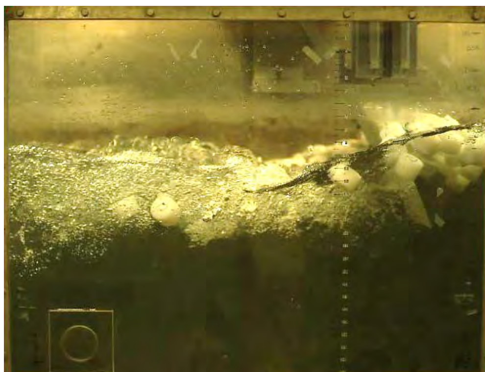
Figure 60. Enlarged Image of the Flow Profile for the Tumblehome Plate at the End of the Ice Section at 7 Hz.
