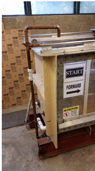
Figure 88. Tow Tank Fill Piping.
