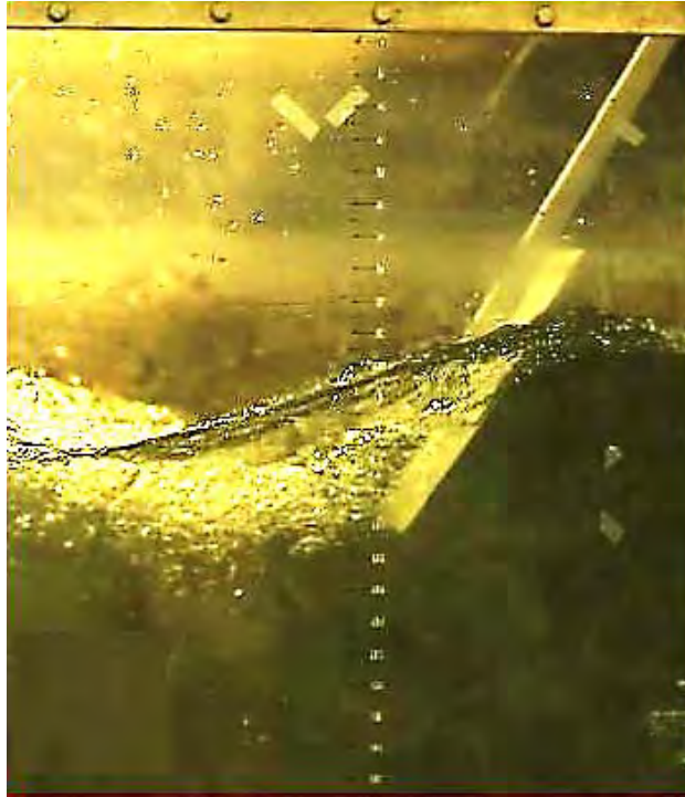
Figure 49. Flow Around Conventional Plate at 9 Hz Exhibiting Full Freeboard.
