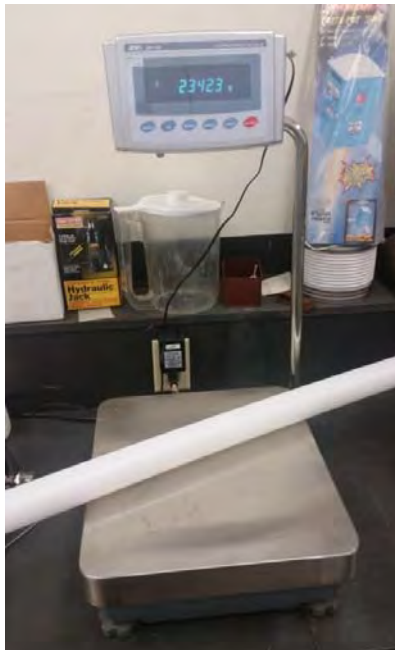
Figure 17. Electric Balance Used in Density Measurements.
