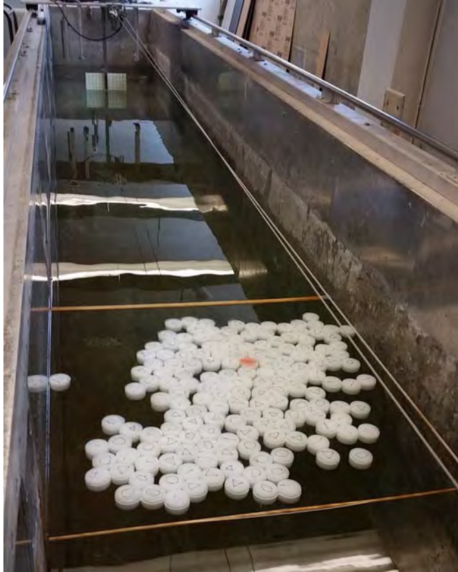
Figure 38. Setup for 50% Capacity Small Ice Trials.
